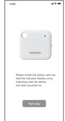
3.3.2 Please make sure the device batteries are installed correctly. When the blue light flashes once, confirm and click "Next Step" to continue.
