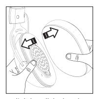
2.Slightly pull the headset and ear pads in the opposite direction to remove the ear pads.
