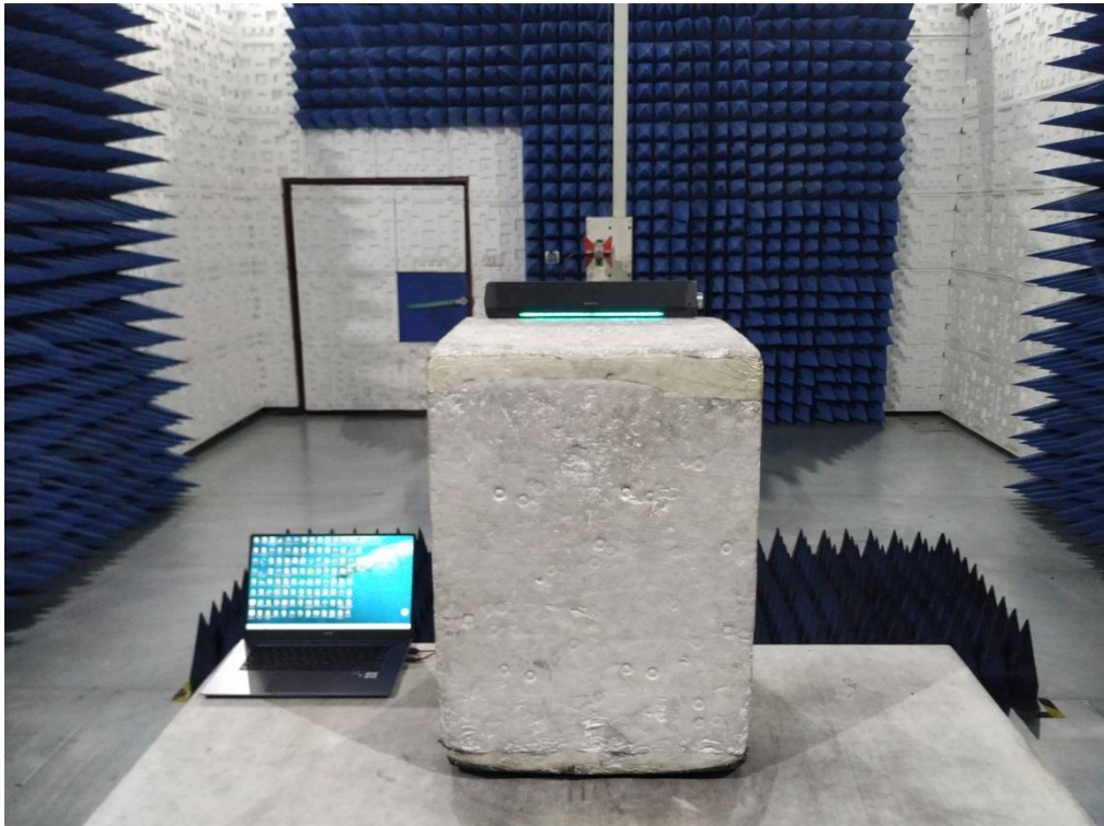
RADIATED EMISSION TEST SETUP ABOVE 1GHz
