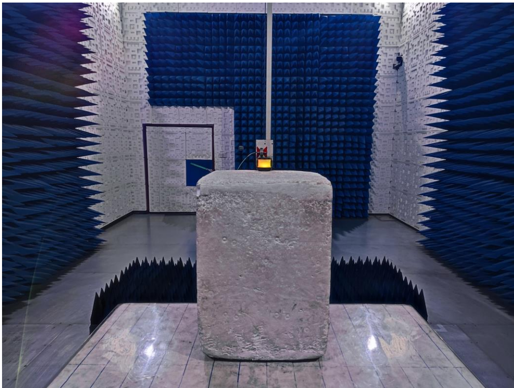
RADIATED EMISSION TEST SETUP ABOVE 1GHz
