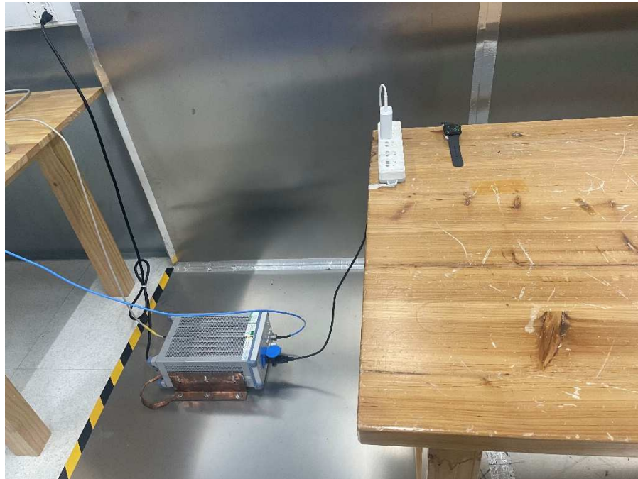
Photograph 3: Set-up photo for Conducted Emission
