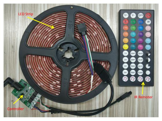
The products are divided into controller, IR remote and LED strip.
