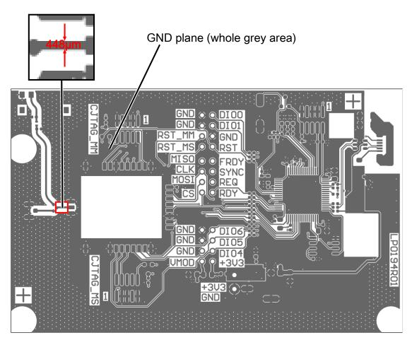
On this layer the module is connected to its periphery. The unused areas are filled with copper that is connected to GND potential. The GND pins of the module are connected directly to this GND plane to receive best possible GND connection with low impedance.
