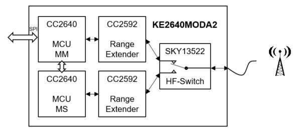
Two RF transceivers of the type CC2640 from Texas Instruments are integrated in this module. It is specified here that only one of the transceivers is used for transmit mode. The second transceiver is only used to support the receive mode of the module. The symmetric RF path design in combination with an RF switch ensures that both transceivers show the same behavior in receive mode. It also ensures that only one RF path can be active at a time.
