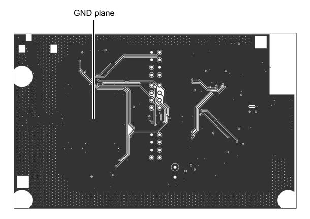
This layer is used for routing signals. Unused areas are filled with GND plane.
