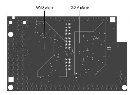
This layer is used for supply planes (3.3V and GND).
