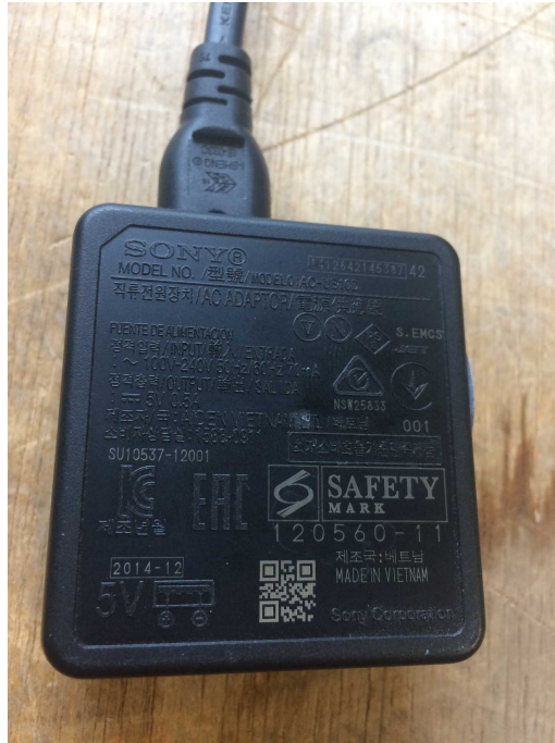
Photo 32: Power supply for AC conducted measurements
