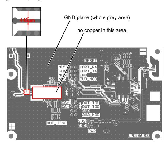
On this layer the module is connected to its periphery. The unused areas are filled with copper that is connected to GND potential. The GND pins of the module are connected directly to this GND plane to receive best possible GND connection with low impedance. There is a copper-free area below the module to avoid short-circuits with non-isolated parts on the bottom side of the module.
