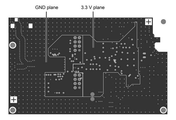
This layer is used for supply planes (3.3V and GND).
