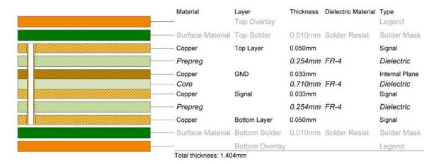
The user can adapt the layer stack-up according to his own requirements. In this case the correct impedance of 50  $\Omega$  has to be ensured. Ideally this is done in cooperation with the selected PCB manufacturer.
