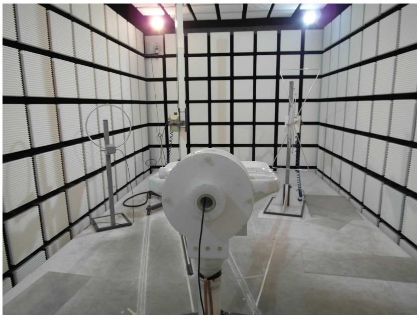
Photo 4: RSE>1GHz / DUT with internal antenna
