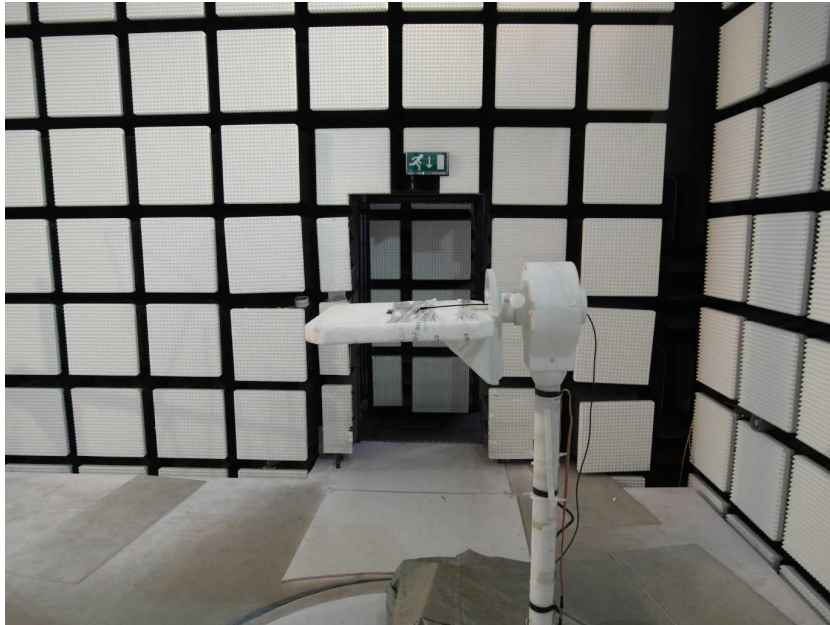
Photo 3: RSE>1GHz / DUT with internal antenna
