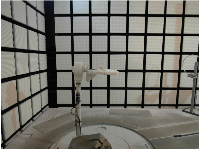
Photo 7: RSE>1GHz / DUT with external antenna
