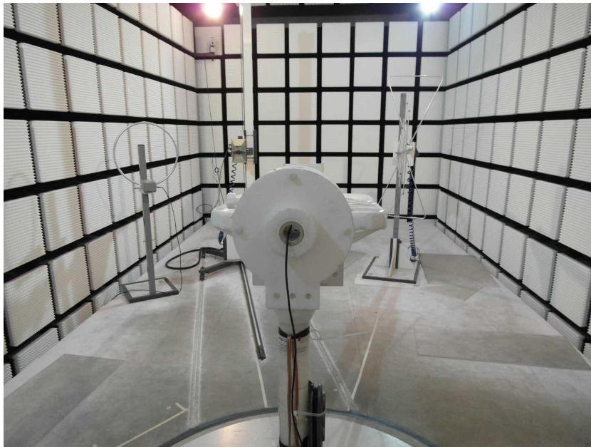
Photo 9: RSE>1GHz / DUT with external antenna
