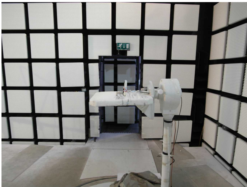
Photo 8: RSE>1GHz / DUT with external antenna
