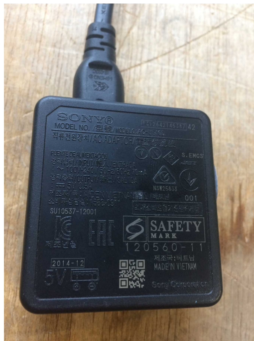
Photo 14: Power supply for AC conducted measurements
