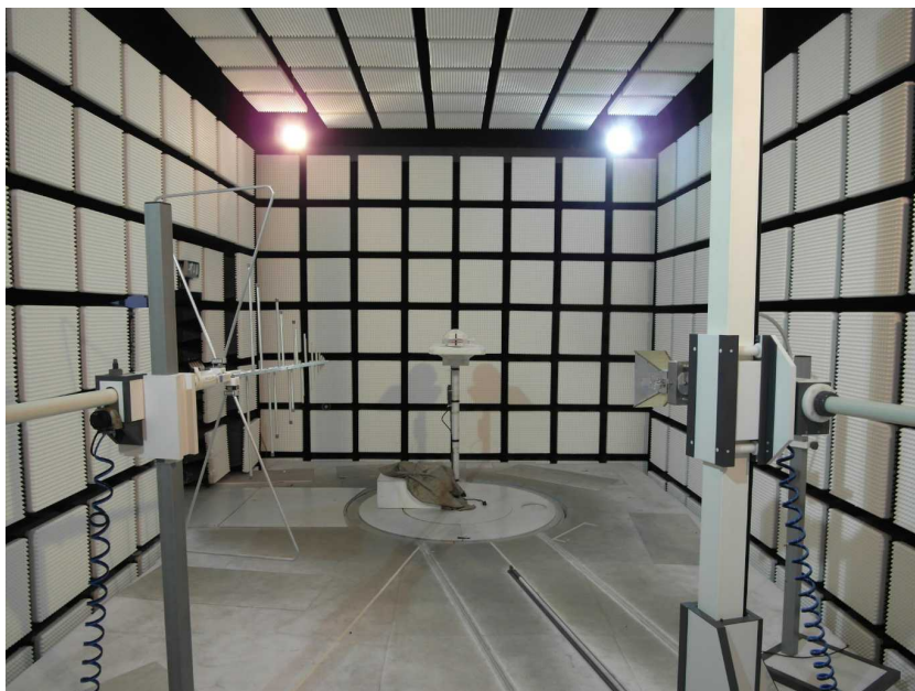
Photo 10: RSE>1GHz / DUT with external antenna
