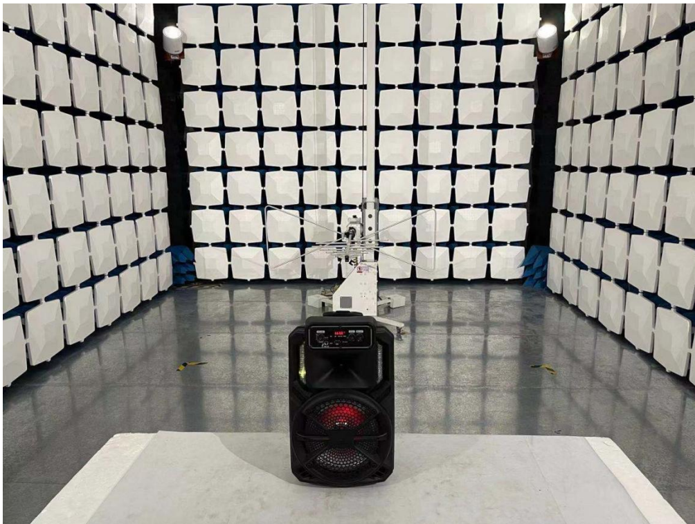
Below 1GHz for radiated emission test setup
