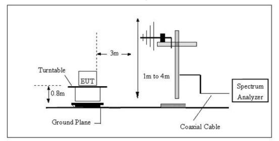
(C) Radiated Emission Test-Up Frequency Above 1GHz
