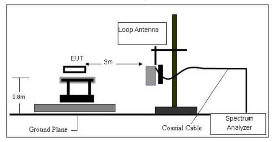
(B) Radiated Emission Test-Up Frequency 30MHz~1GHz
