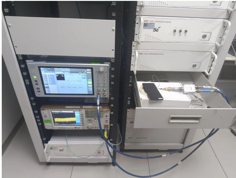
RF Conducted Test setup (GSM/WCDMA/LTE)
