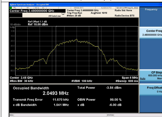
Test Mode:GFSK (LE 2Mbps) 2480MHz
