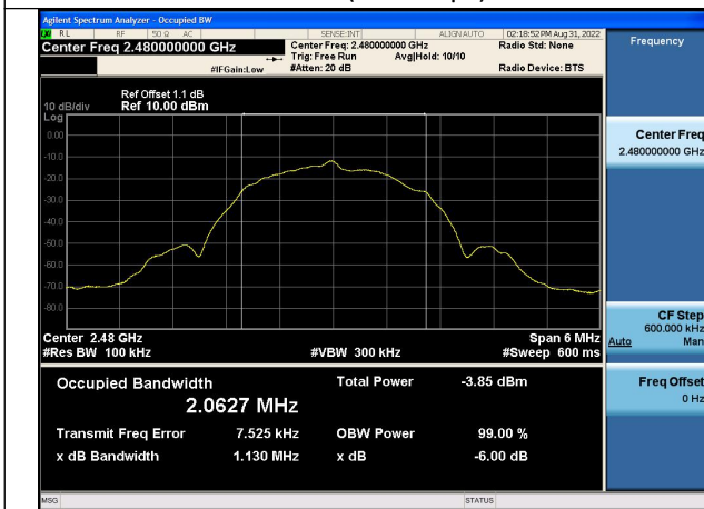
Test Mode:GFSK (LE 2Mbps) 2480MHz
