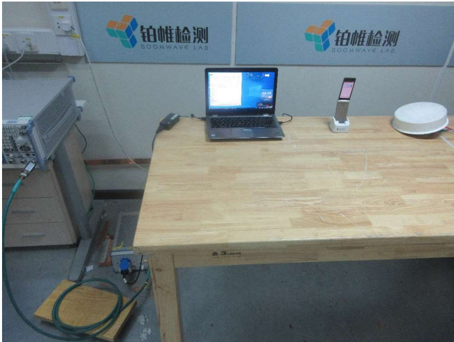
Conducted Emission 150kHz-30MHz (Front view) – Mode 5
