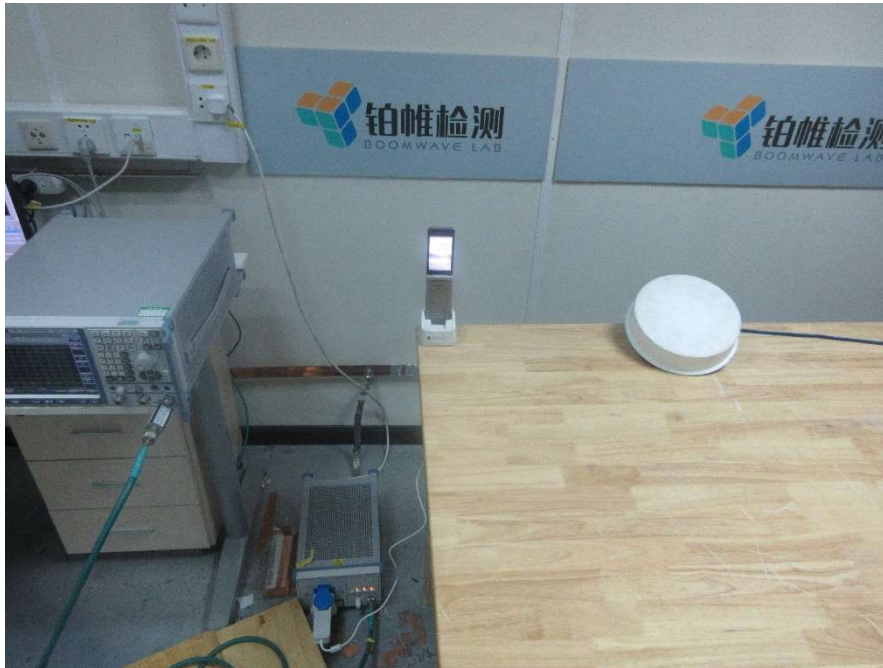
Conducted Emission 150kHz-30MHz (Front view) – Mode 2
