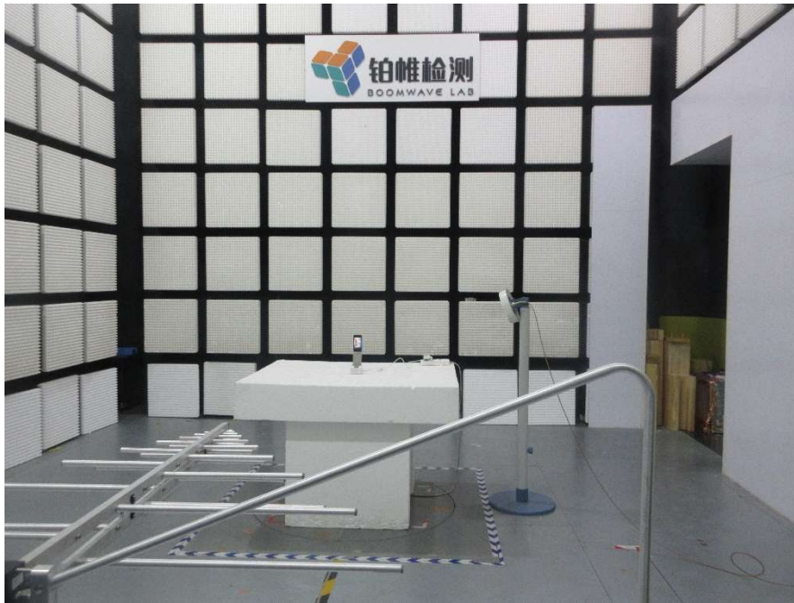
Radiated Emission 30MHz-1GHz – Mode2
