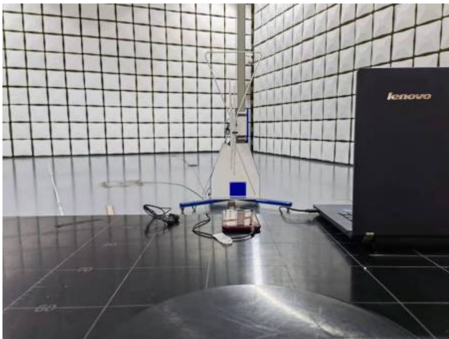
Radiated Emissions Test Setup (with laptop) (30-1000MHz)
