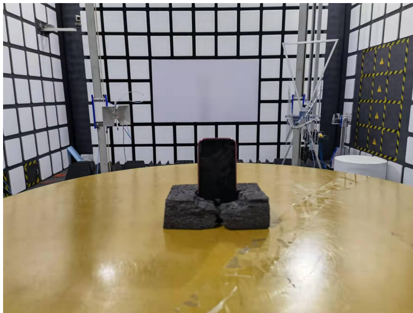
Spurious Radiated Emissions Test setup
