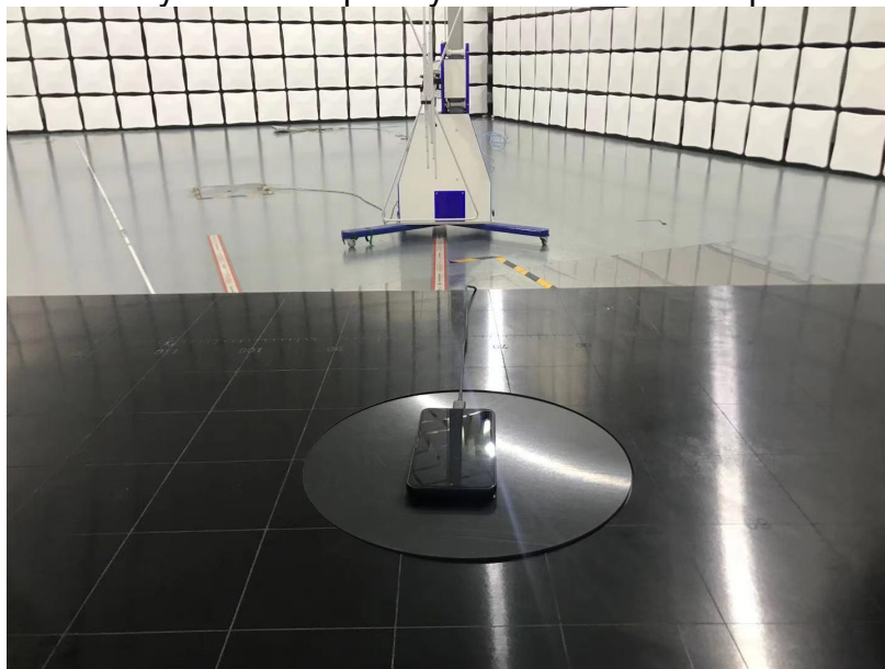
Dynamic Frequency Selection Test setup
