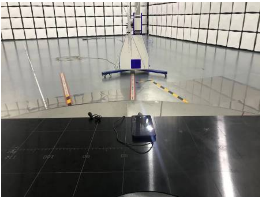
Radiated Emissions Test Setup (30-1000MHz)
