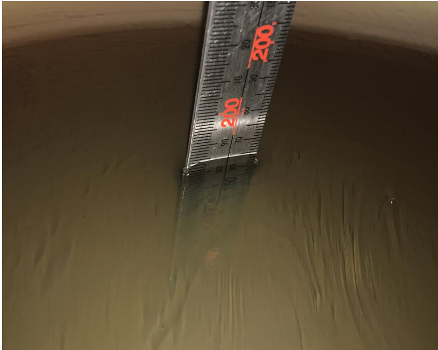
Liquid depth for SAR Measurement
