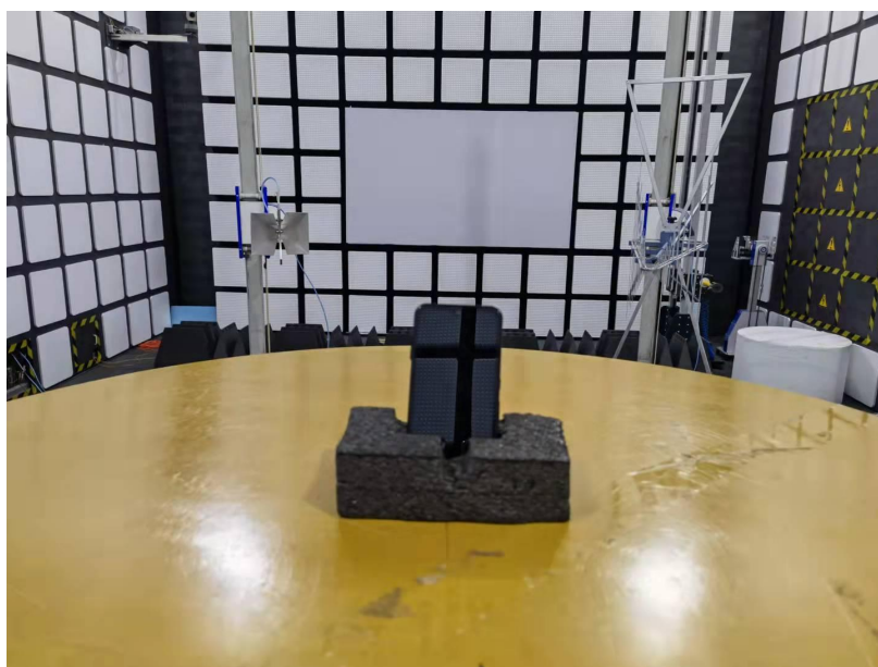
Spurious Radiated Emissions Test setup
