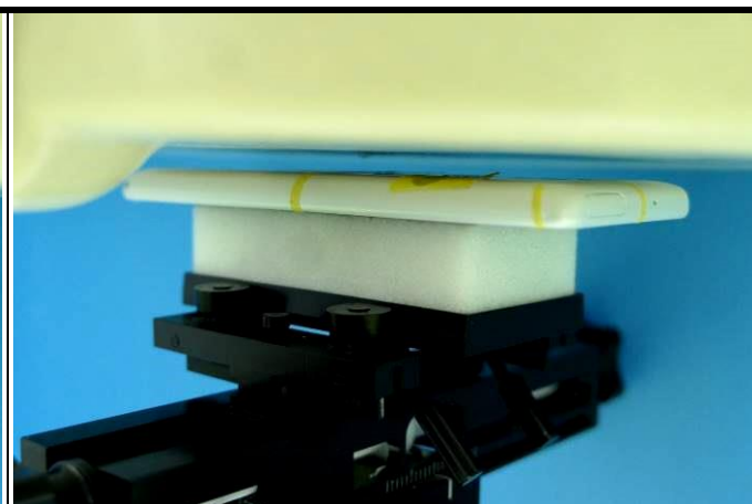
Hotspot - Rear Face of EUT at 5 mm
