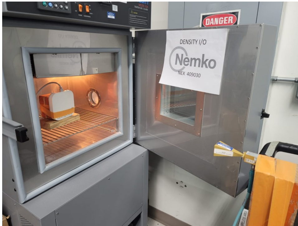
Figure 5 – Frequency stability test setup
