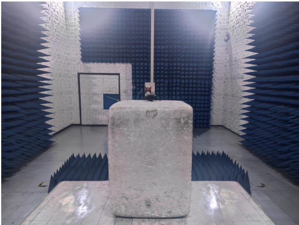
RADIATED EMISSION TEST SETUP ABOVE 1GHz
