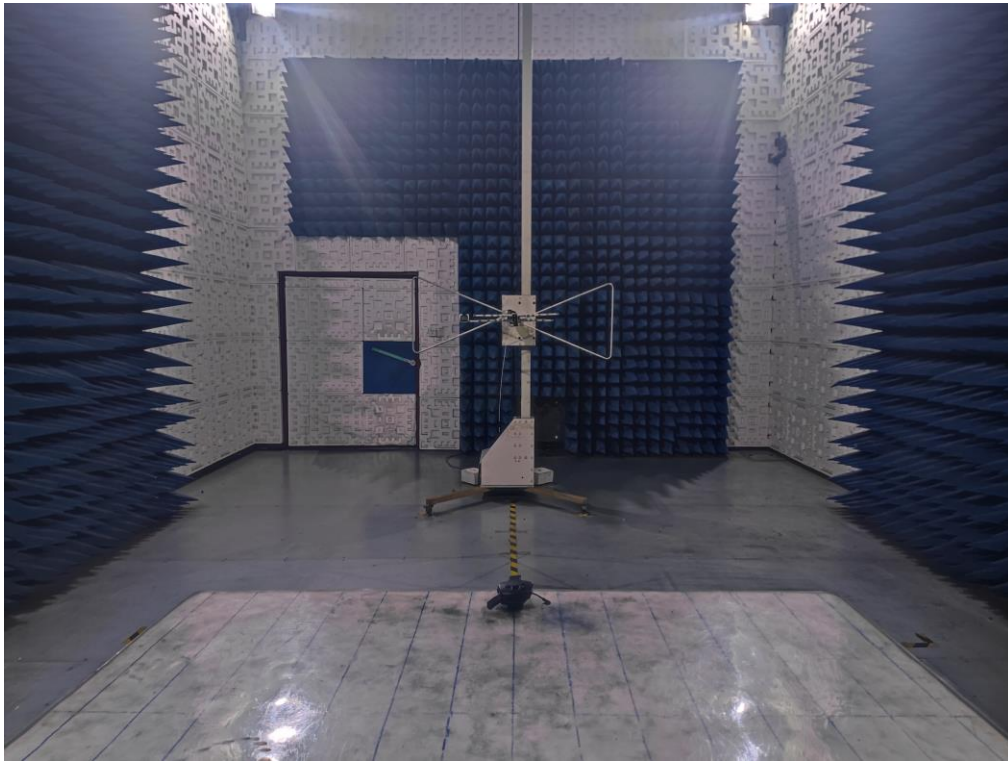
RADIATED EMISSION TEST SETUP ABOVE 1GHz
