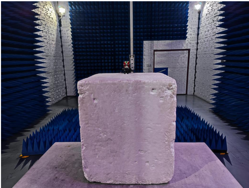
RADIATED EMISSION TEST SETUP ABOVE 1GHz
