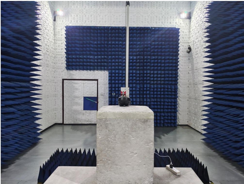
RADIATED EMISSION TEST SETUP ABOVE 1GHZ
