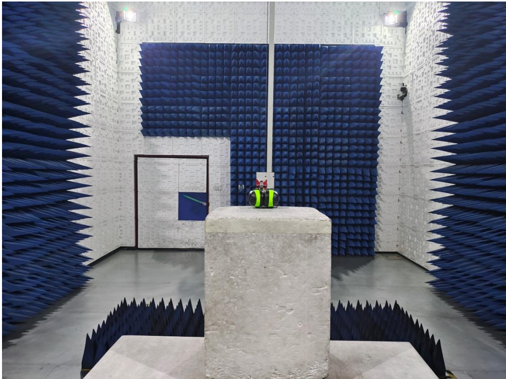
RADIATED EMISSION TEST SETUP ABOVE 1GHz
