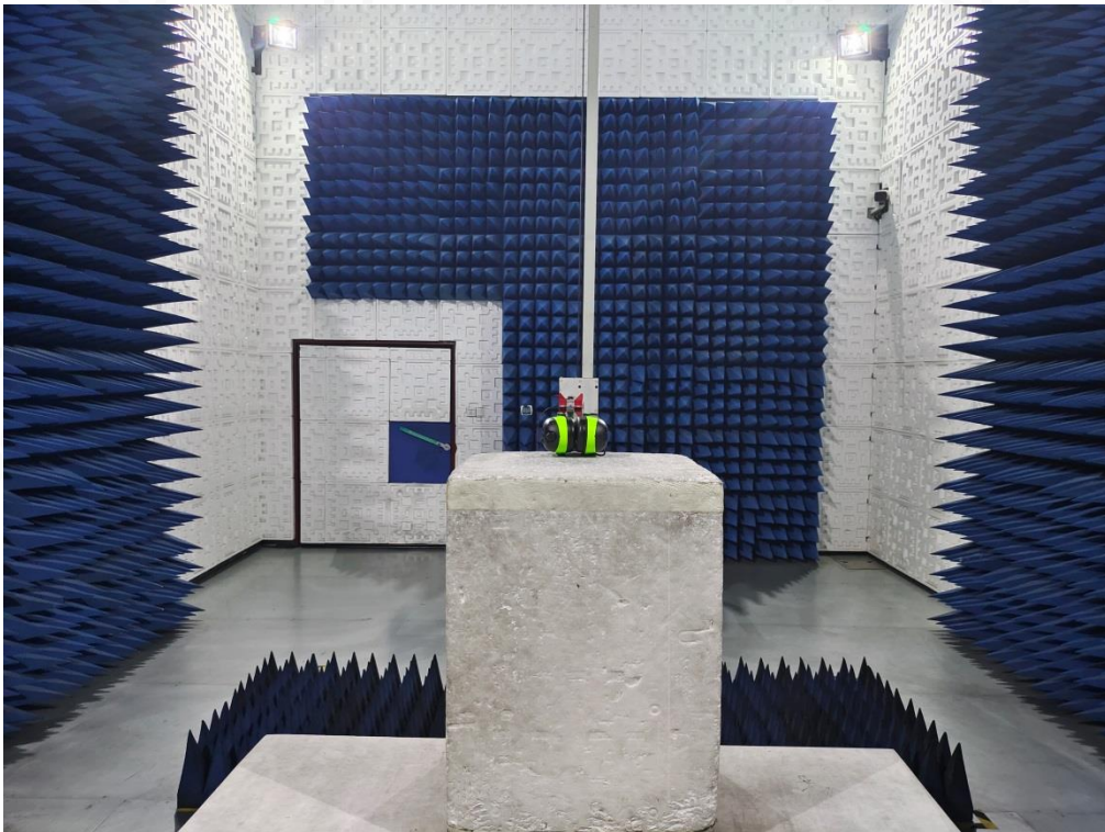
RADIATED EMISSION TEST SETUP ABOVE 1GHZ
