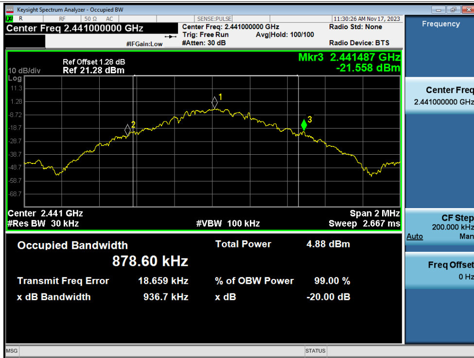
-20dB Bandwidth NVNT 1-DH5 2441MHz Ant1
