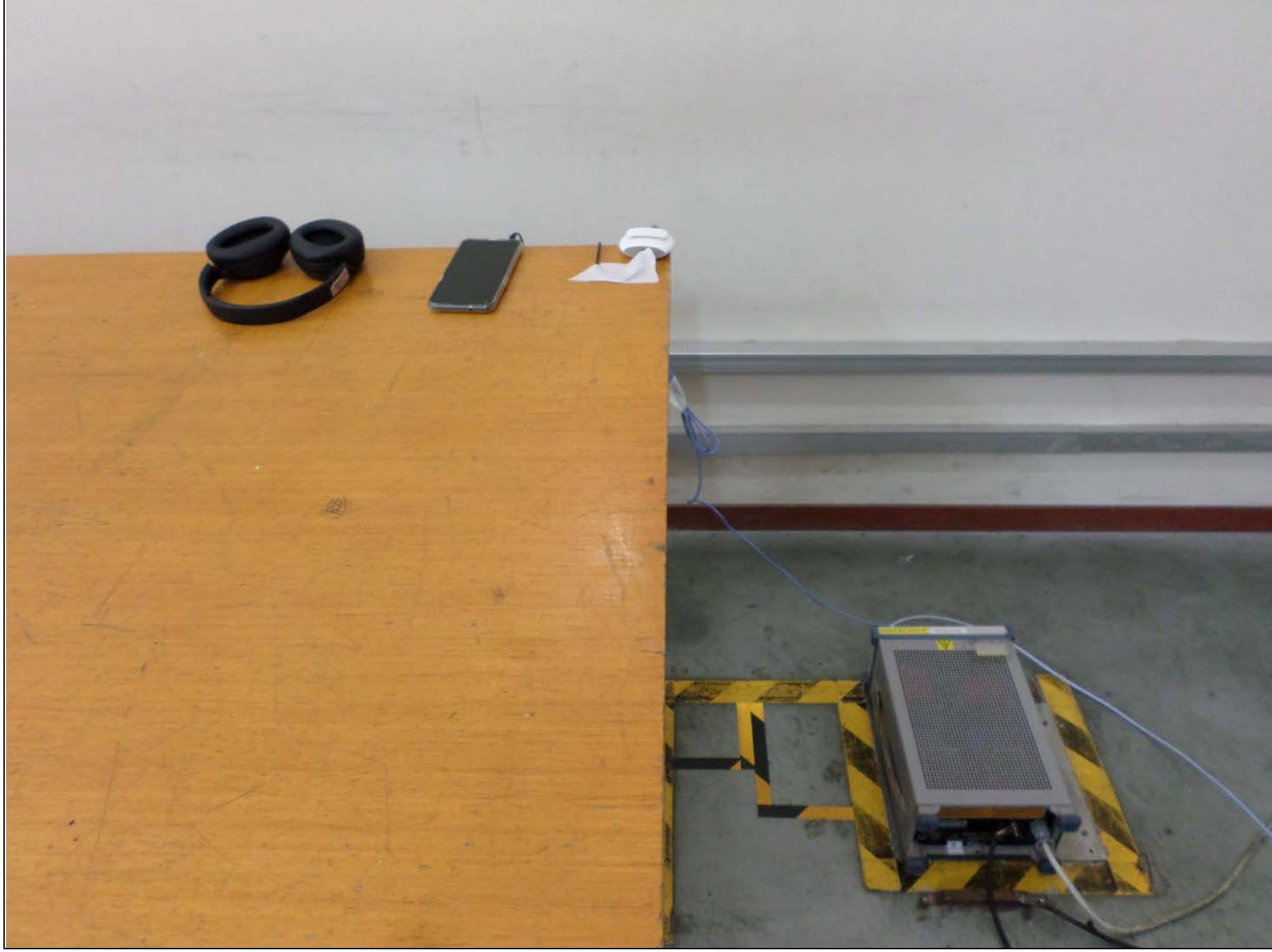
Continuous Conducted Emission at main _ Front
