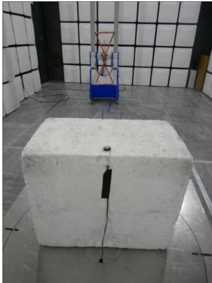
Figure 60 - Test Setup - 30 MHz to 1 GHz - X Orientation
