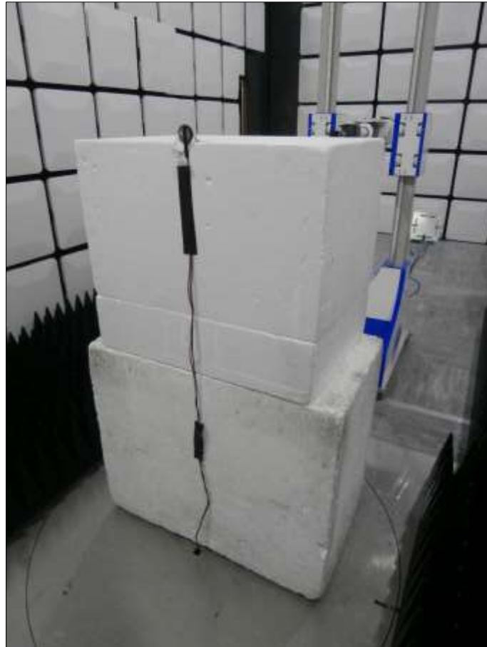
Figure 68 - Test Setup - 18 GHz to 25 GHz - Z Orientation
