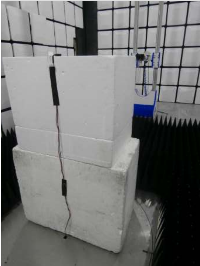
Figure 63 - Test Setup - 1 GHz to 18 GHz - X Orientation
