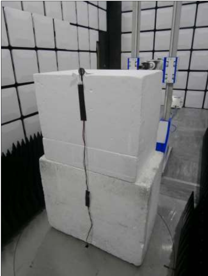
Figure 67 - Test Setup - 18 GHz to 25 GHz - Y Orientation
