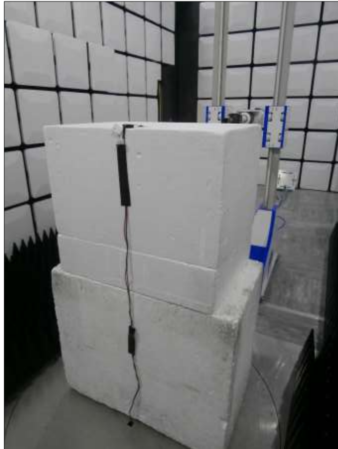
Figure 66 - Test Setup - 18 GHz to 25 GHz - X Orientation
