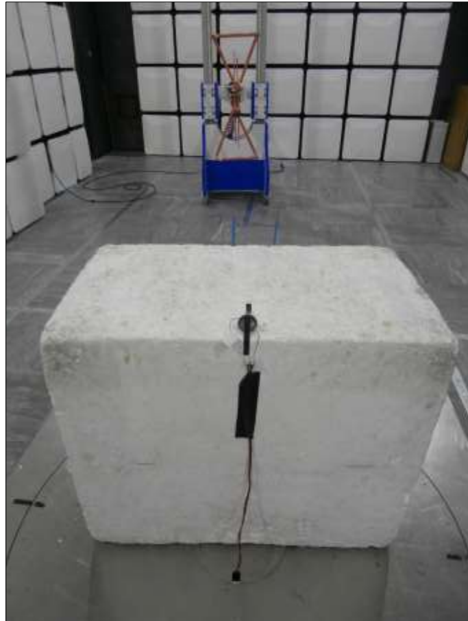
Figure 62 - Test Setup - 30 MHz to 1 GHz - Z Orientation
