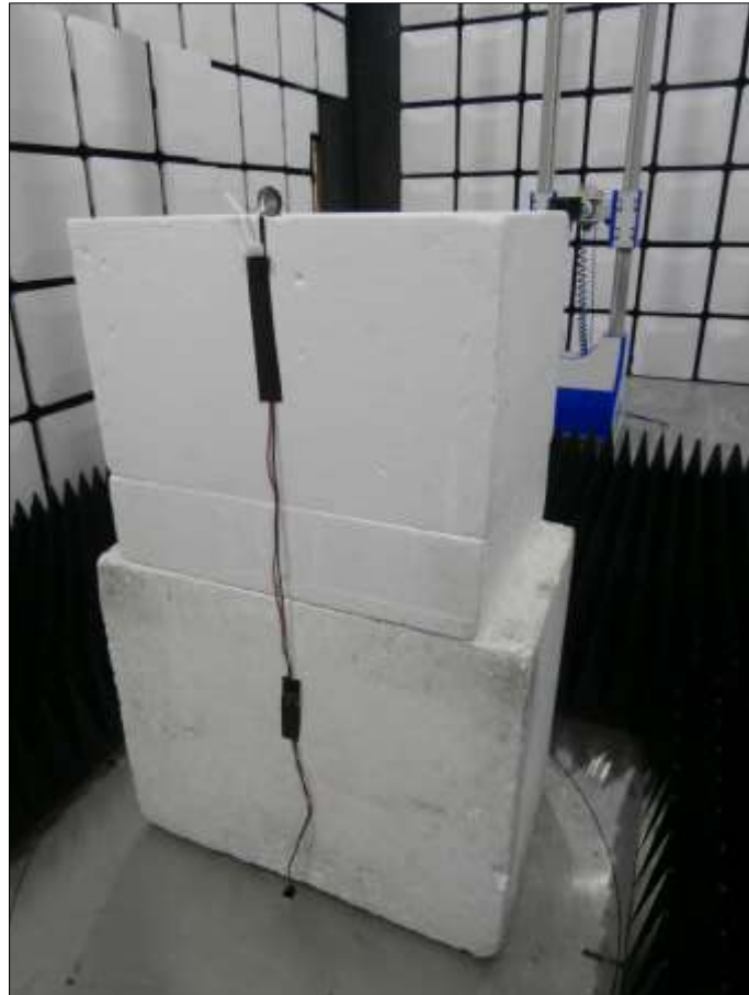
Figure 65 - Test Setup - 1 GHz to 18 GHz - Z Orientation
