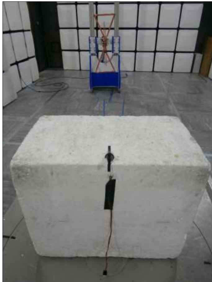
Figure 61 - Test Setup - 30 MHz to 1 GHz - Y Orientation
