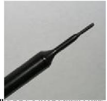
Figure 4.4 EX3DV4 E-field Probe
