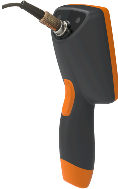
Fig. 4 – Connecting the charging cable to the charging port of the Smart Probe.
