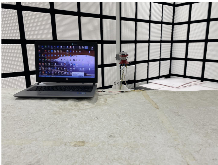
Radiated spurious emission Test Setup-3(Above 1GHz)
