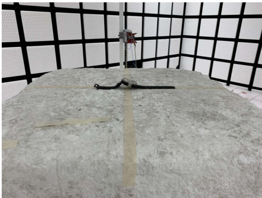
Radiated spurious emission Test Setup-2(Above 1GHz)
