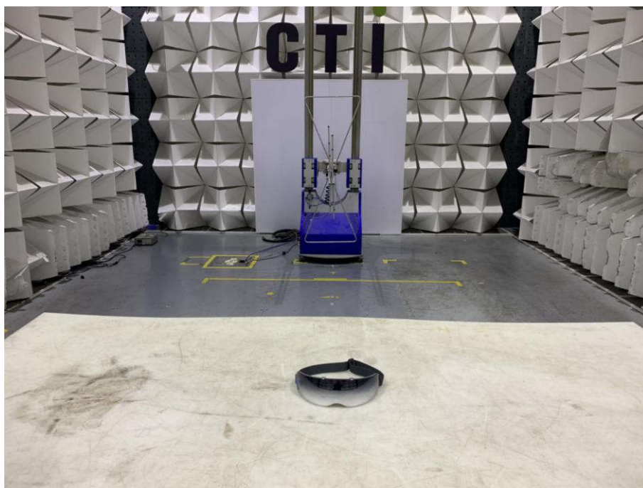
Radiated spurious emission Test Setup-1(Below 1GHz)
