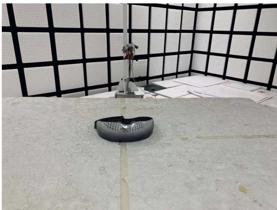
Radiated spurious emission Test Setup-2(Above 1GHz)
