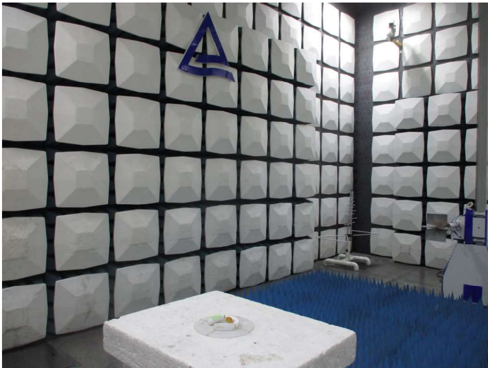
Photograph 2: Set-up for Radiated Spurious Emission, 1GHz - 18GHz
