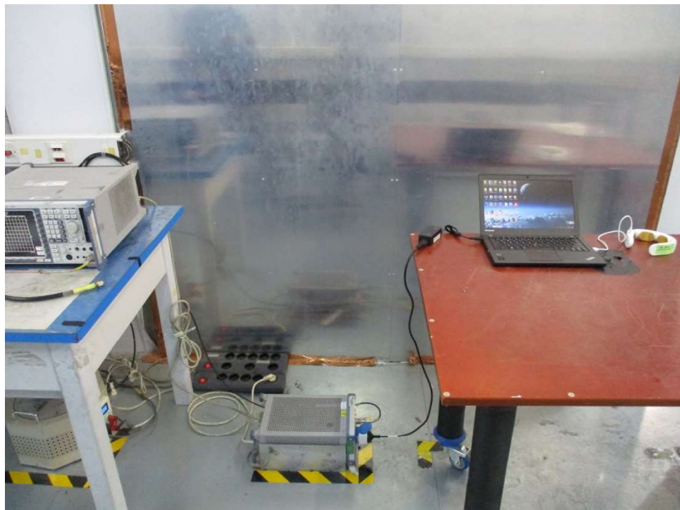
Photograph 4: Set-up for Conducted Emission on AC Mains
