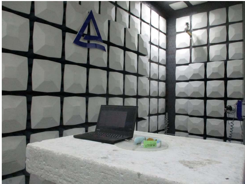
Photograph 4: Set-up for Conducted Emission on AC Mains
