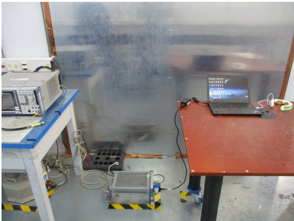
Photograph 4: Set-up for Conducted Emission on AC Mains
