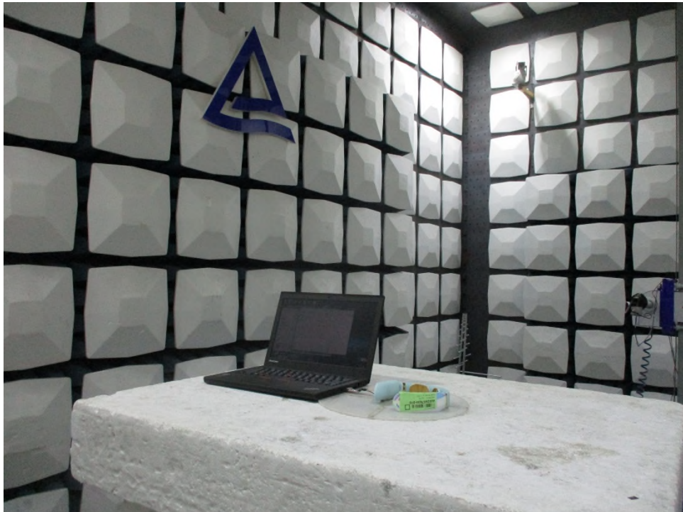
Photograph 4: Set-up for Conducted Emission on AC Mains
