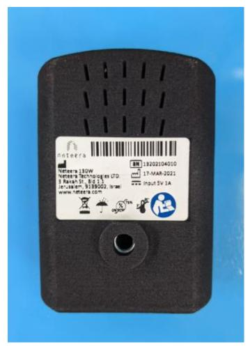
Label with **FCC ID: 2AYVO-NETEERA1301** will be located at the bottom part of the unit's shell, on the motor cover. The statement according to FCC part 15 §15.19(a)(3).
