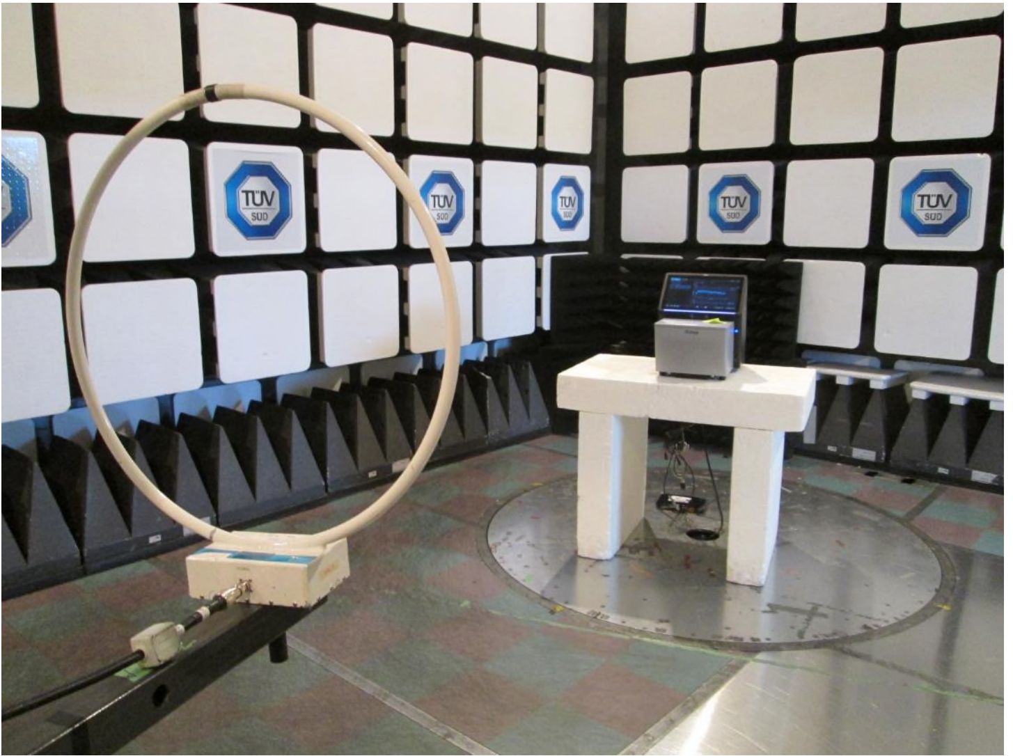
Test setup photo 1 Radiated measurements, 9 kHz – 30 MHz
