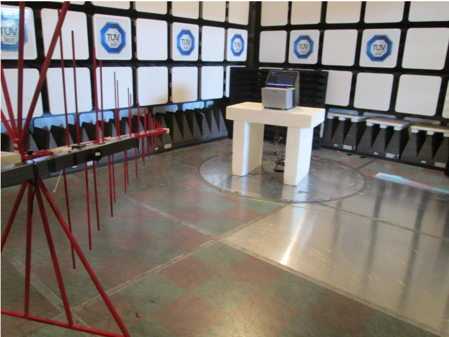
Test setup photo 2 Radiated measurements, 30 MHz – 1 GHz
