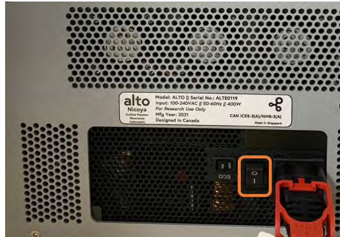
Figure 4.18: Instrument is turned on by toggling the AC power switch with the I position depressed.
