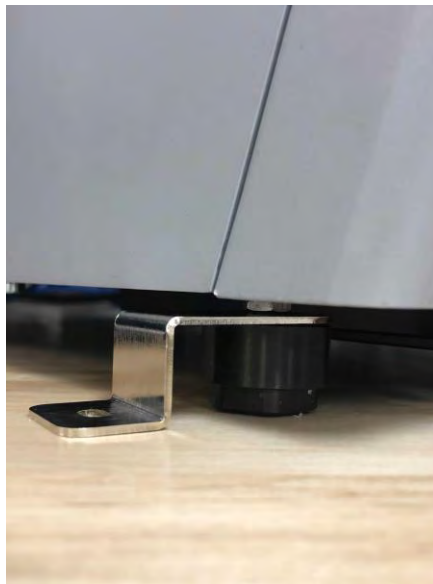
Figure 4.11: Instrument foot with a table mounting bracket installed.
