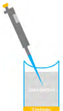
Figure 5.33: Lower the pipette tip into the cartridge fluid without touching the bottom of the cartridge or electrode.
