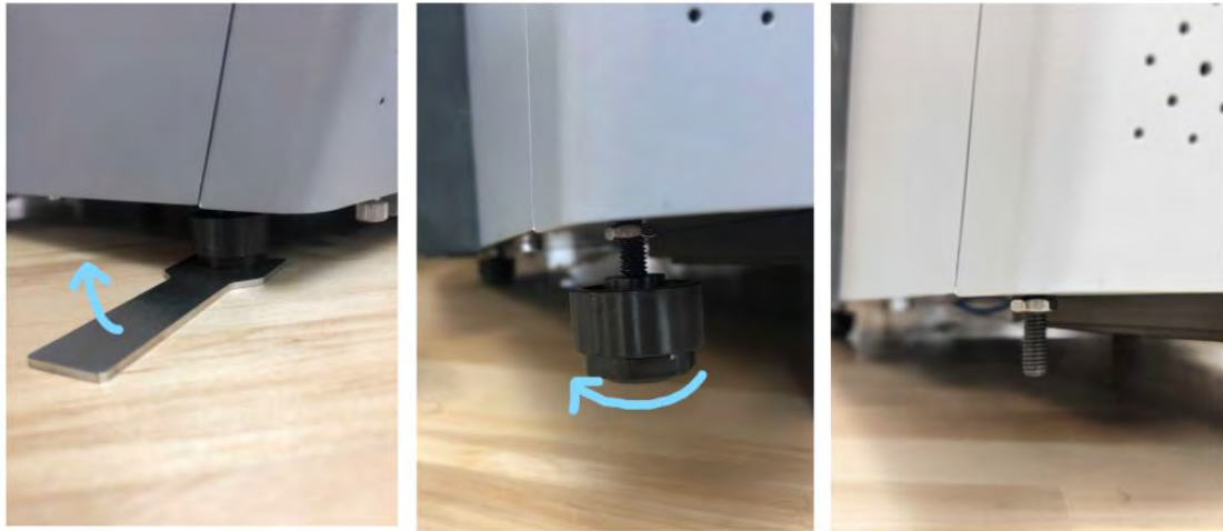
Figure 4.10: The process of unscrewing the instrument foot.
