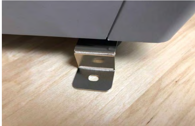
Figure 4.12: Table mount bracket before being attached to the lab bench.
