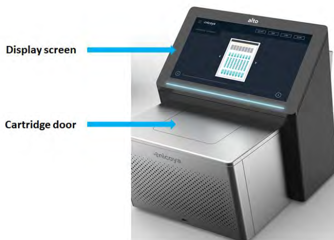
Figure 3.1: Alto instrument and components.
