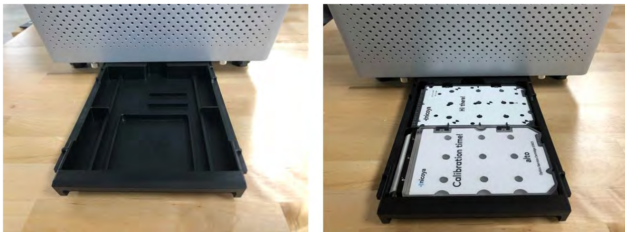
Figure 3.5: Drawer under the instrument for storing the QC cartridge, OSC cartridge and accessories.
