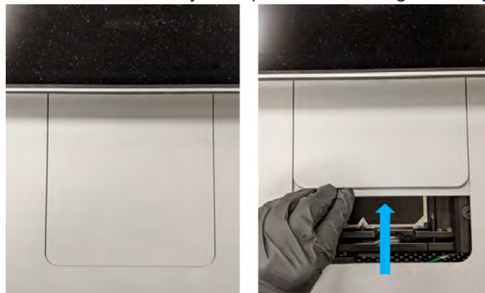
Figure 4.5: Push the cartridge door open manually to expose the cartridge loading bay.
