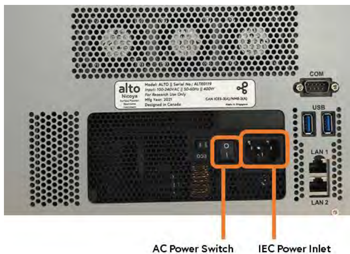
Figure 4.16: AC power switch and IEC power inlet location and configuration prior to attaching the power cable.
