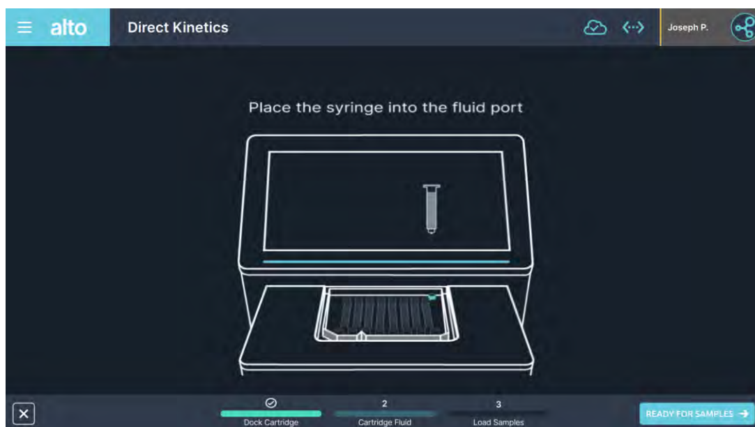
Figure 5.28: Cartridge fluid syringe loading into the fluid port on the cartridge.
