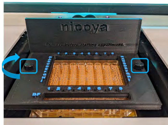
Figure 5.36: Securing the pipette guide onto the cartridge loading bay with the hand screws.
