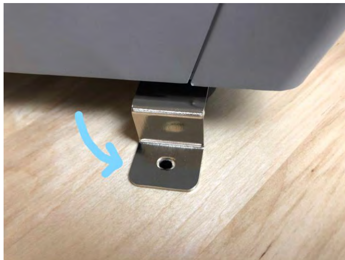
Figure 4.13: Ensure the table mount bracket is directly over the drilled hole.
