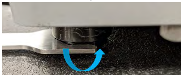
Figure 4.8: Turn the foot counterclockwise using the foot wrench and monitor the bubble level.
