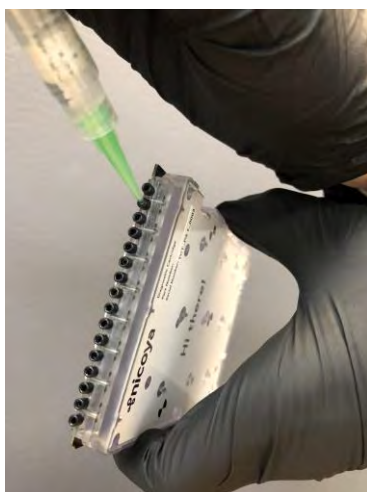
Figure 5.14: Optical gel application for the QC cartridge.
