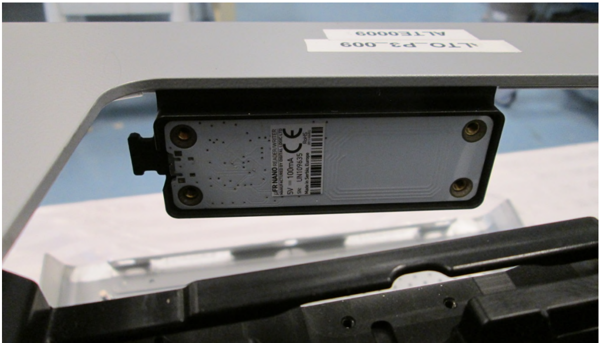
EUT – Internal view 9 NFC board within compartment
