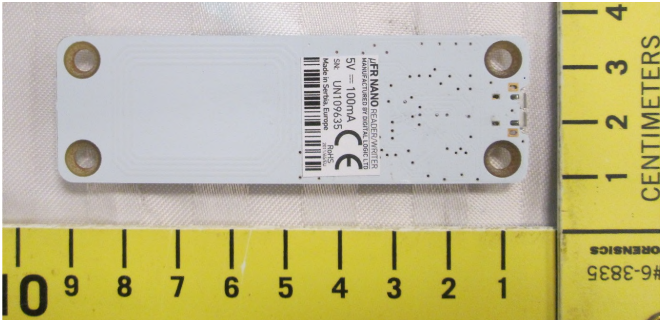
EUT – Internal view 10 NFC board, side 1
