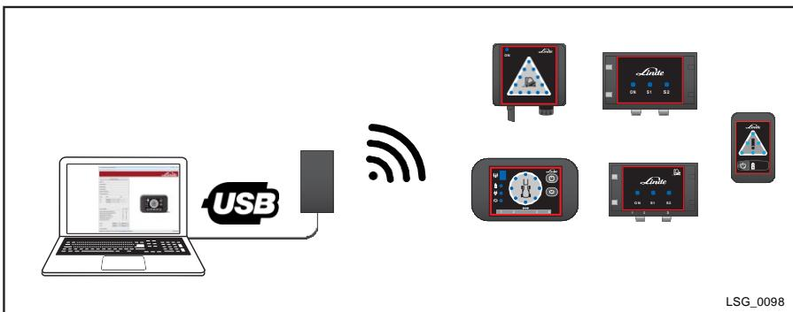
Use the additional USB-Cable to connect the programmer to your computer. With the software tool "Wireless Flasher", the programmer enables you to send new firmware to the devices. Furthermore, the provided configuration tool enables the service technician to configure the signaling zones.
