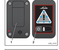
➤ Attach the Distance Beeper to the outside of your workwear using the clip (1).
