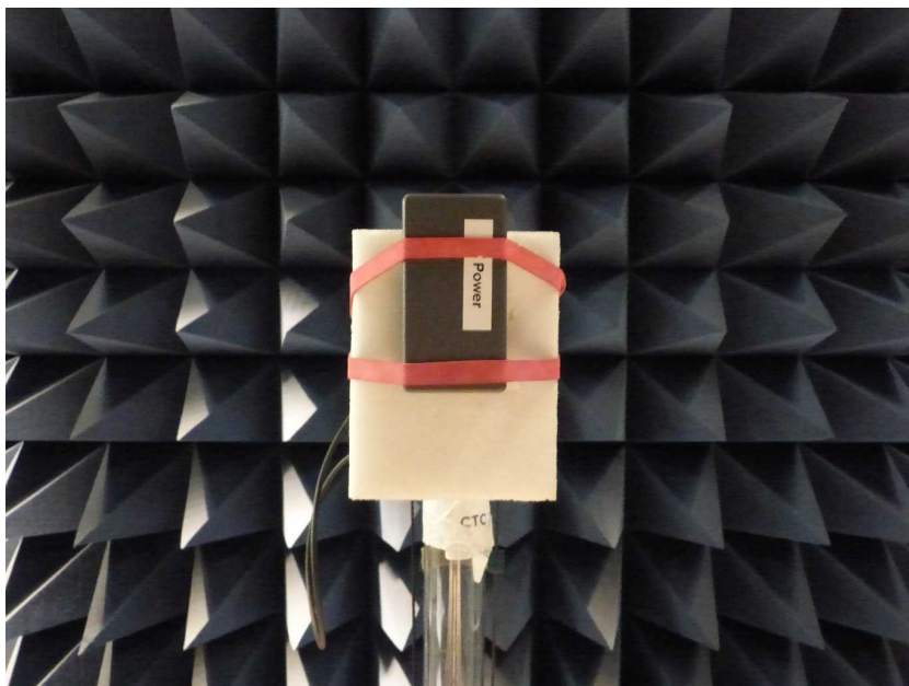
Photo 8: EUT at the fully anechoic chamber (1-18 GHz)
