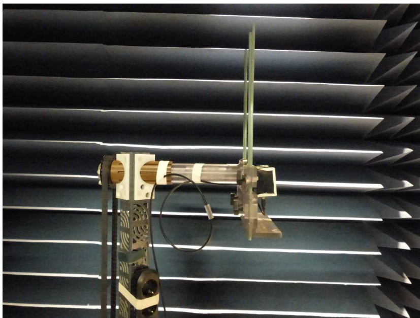
Photo 6: EUT at the anechoic chamber (1-18 GHz)
