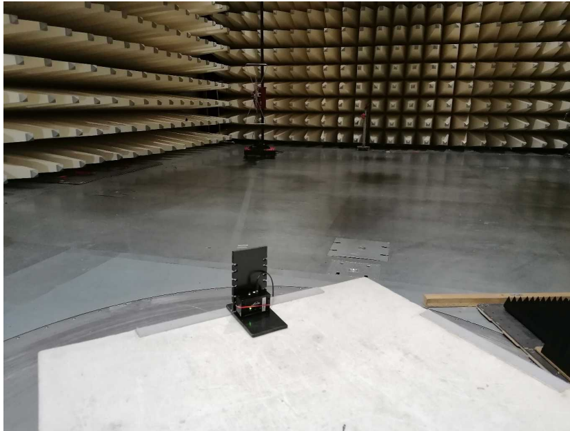
Photo 1: EUT at the semi-anechoic chamber
