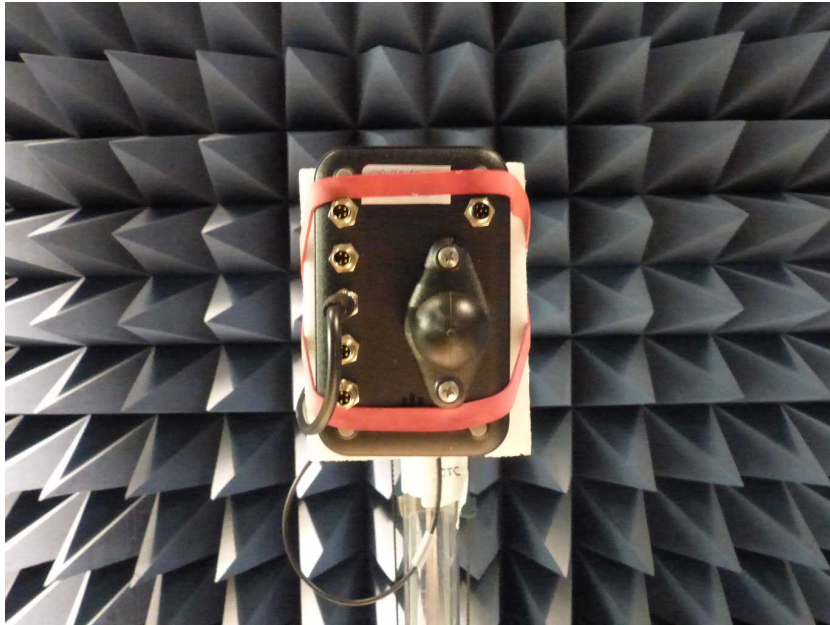
Photo 7: EUT at the anechoic chamber (1-18 GHz)
