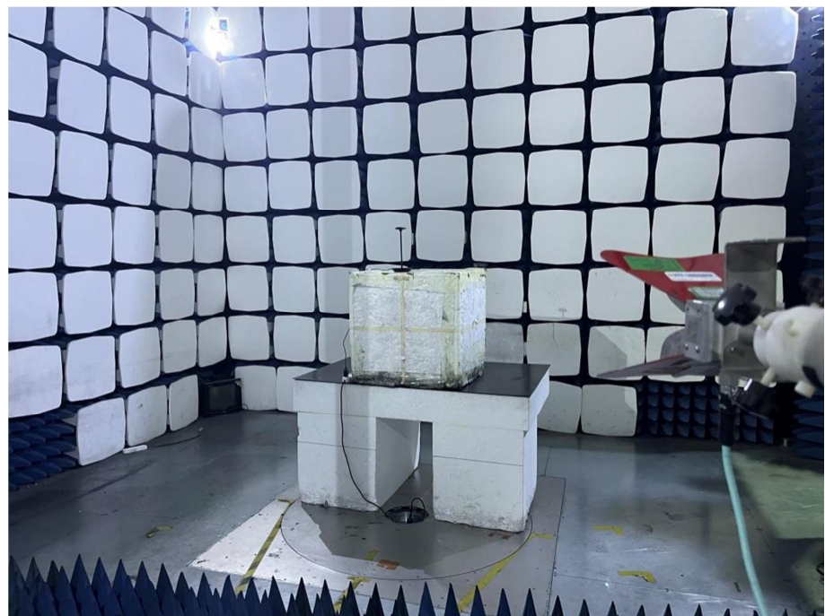
Radiation Emission Test Setup (1GHz to 18GHz)
