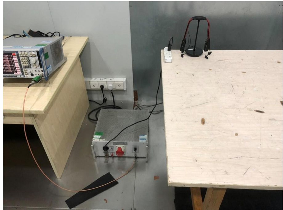
Conducted Emission Test Setup
