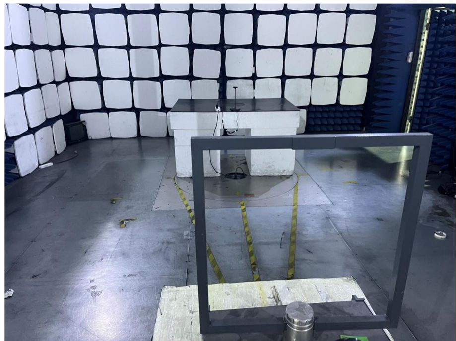
Radiation Emission Test Setup (Below 30MHz)
