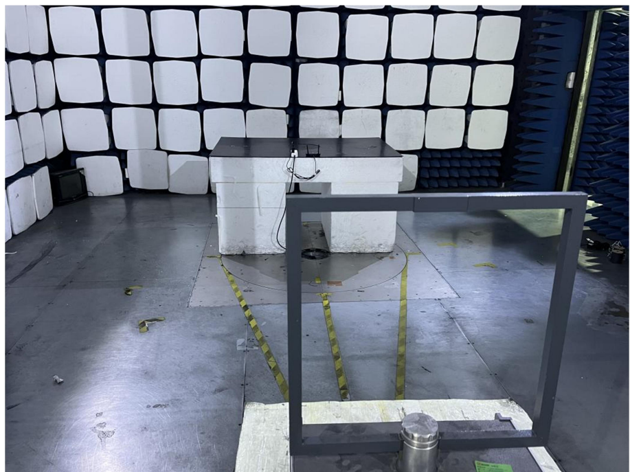
Radiation Emission Test Setup (Below 30MHz)
