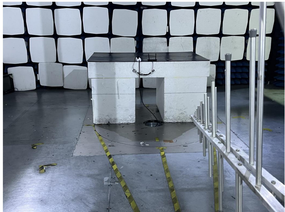
Radiation Emission Test Setup (30MHz to 1GHz)
