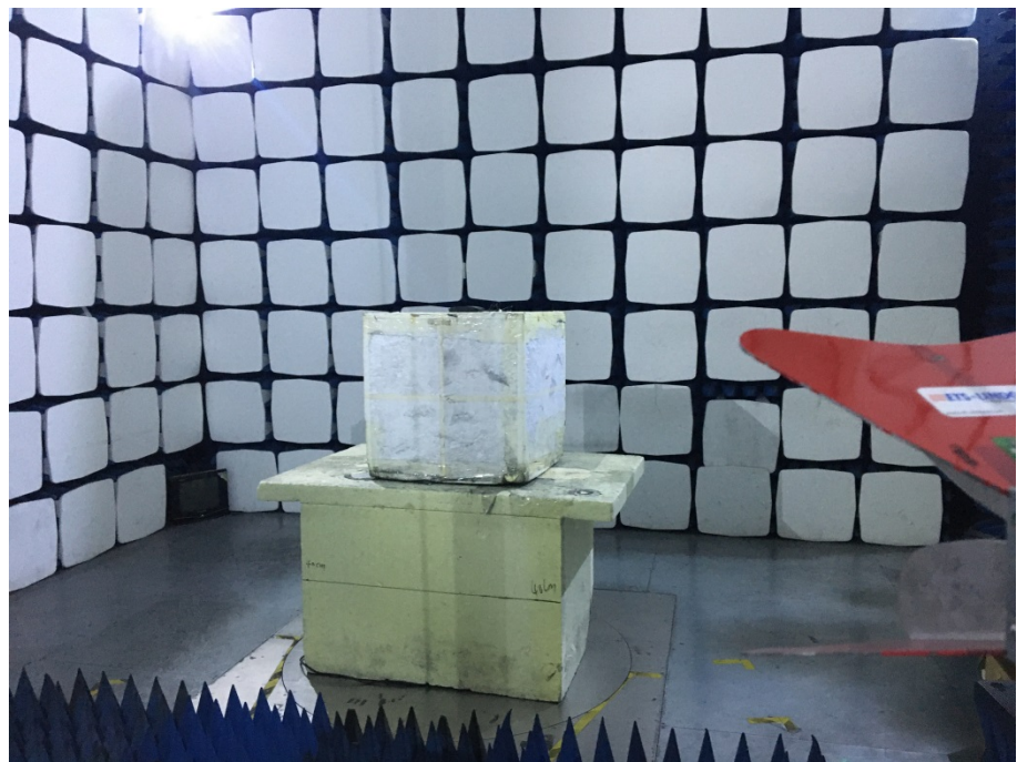
Radiation Emission Test Setup (1GHz to 18GHz)
